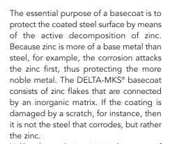
Unlike electroplating, it is in the nature of the zinc flake application that no hydrogen-induced cracking corrosion occurs (hydrogen embrittlement), which is particularly important in the case of screws and high-tensile steel.
